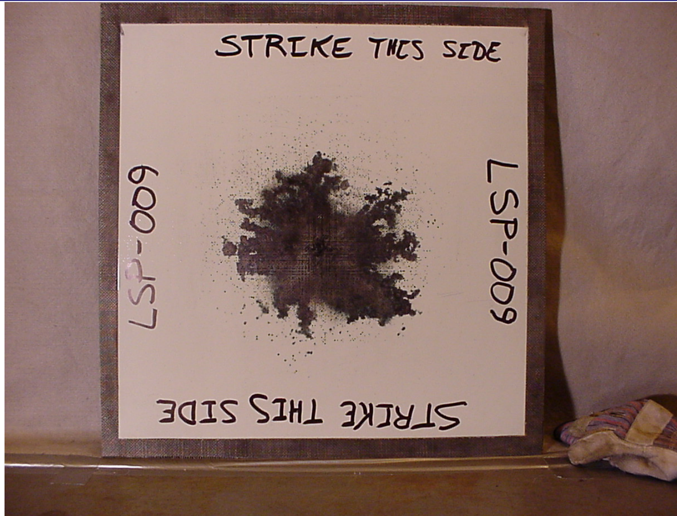
LSP-009, Interwoven Phos-Bronze mesh, Aramid core, after Zone 1A strike
