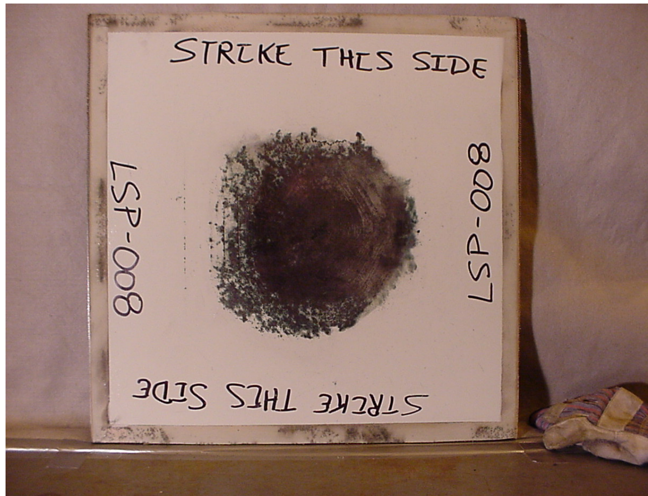
LSP-008, Copper mesh, aramid core, after Zone 1A strike
