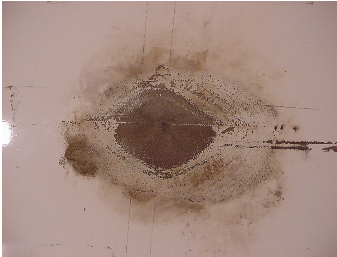
Panel 009, butt splice using aluminum mesh
